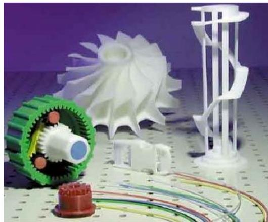
Rapid prototypes created using FDM. (PERIDOT, Inc. Rapid Prototyping)
