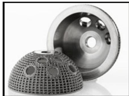
Titanium Medical Implant made by EBM
