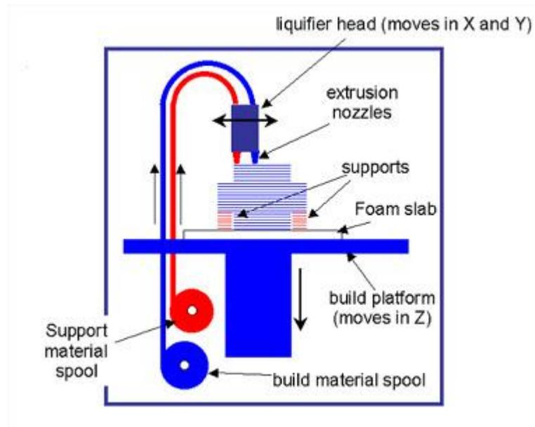
Fused Deposited Modeling (FDM) process schematic.
