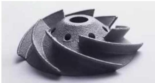
Impeller made using EBM
