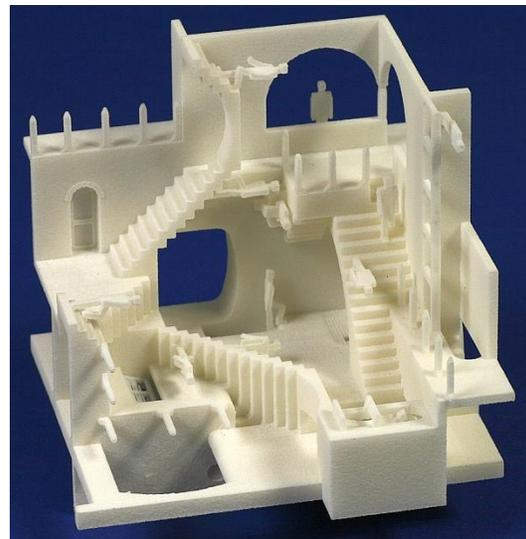
Escher's Relativity, made of nylon by selective laser sintering on a 3D printing machine. (Oded Fuhrmann and Gershon Elber, Technion – Israel Institute of Technology)
