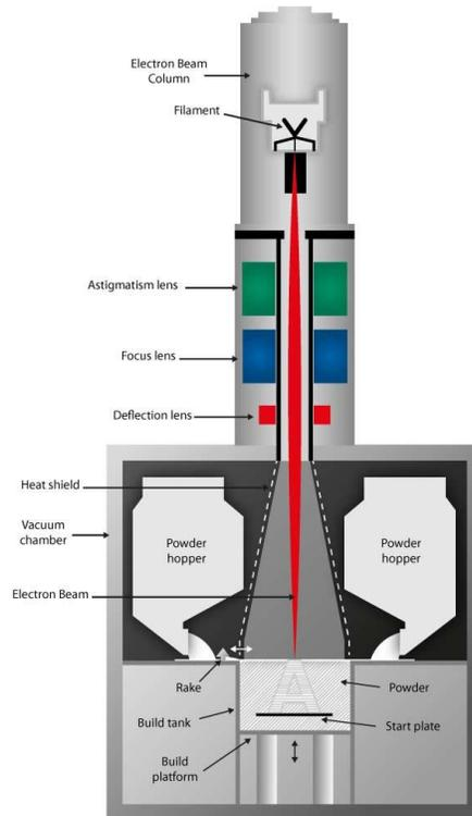
Electron Beam Melting (EBM) process schematic (Arcam AB Additive Manufacturing)
