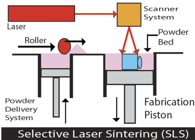
Selective Layer Sintering process schematic.
