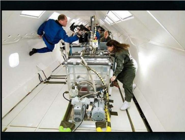
NASA low gravity parabolic flight testing of Made in Space 3-D printer.
